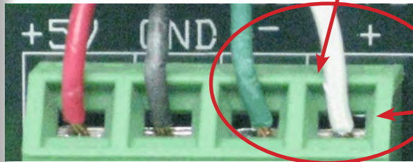
Enlarged view of Thermostat block wiring
